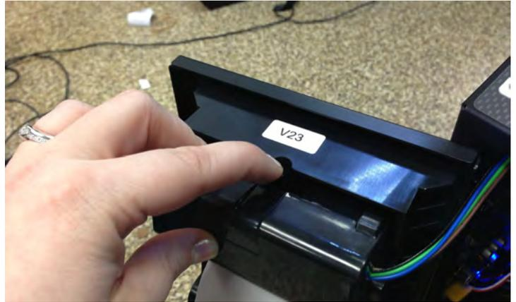
Turn the lever to open the print head, exposing the rollers.
