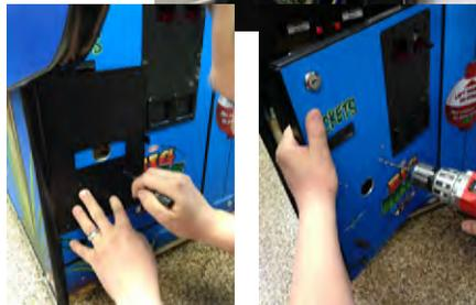
Mark 2-4 of the holes in the back plate onto the cabinet, and drill out with a 3/16" drill bit.
