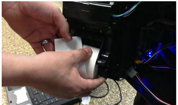
Feed the trimmed end of the paper through the printer as shown.
