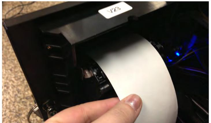
The paper should automatically feed into position, cut and print the Evolve logo. If not, try loading the paper again.
