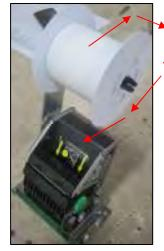
Note: Paper must feed under holder and into printer
