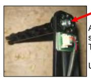
Attach the core holder to the arm using the large screw provided.
