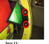
Step 11: Move around to the back of the game. Begin to slide the wheel assembly straight back.
