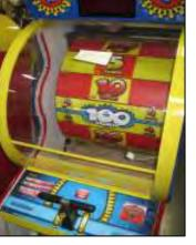
Step 9: Remove the arrow assembly from the game. Be careful not to damage the sensor when removing the arrow.
