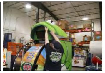
IF YOU CHOOSE TO USE THE BOBBER ASSEMBLY, RUN THE PIPE AND CABLES DOWN THROUGH THE FISH HEAD. THERE IS A WOODEN HOLDER THAT THE PIPE WILL SIT IN BEHIND THE MONITOR.
