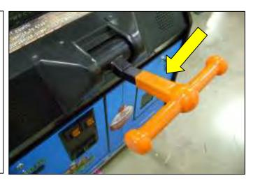
FROM INSIDE THE GAME, INSERT THE BOLT THROUGH THE BRACKET ARM AND HANDLE. SECURE USING THE LOCKNUT.
