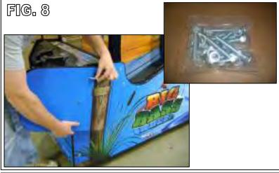
Place the bolt through the hole in the guard and into the cabinet. From inside the cabinet secure the bolts using the flat washer, split washer, and locknut, fig. 9.
