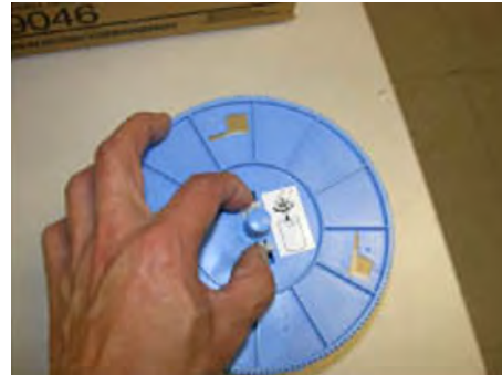
Squeeze the two notches towards center.
