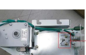
(2) Loosen 3 the bolts and nuts of belt adjustment BKT of FRA to move.
