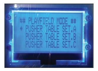
Then, push select button among SET UP buttons and perform Perform by pushing Select button as OPERATION MENU / PLAYFIELD SETUP / PUSHER TABLE SET.A in order.
