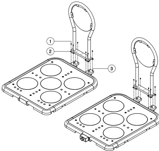
1. Attach ② REAR PIPE to ③ ASS'Y PIPE Fix Bracket by using ① M6x16L Bolts. (for both Left/Right, 16 Bolts in total)
