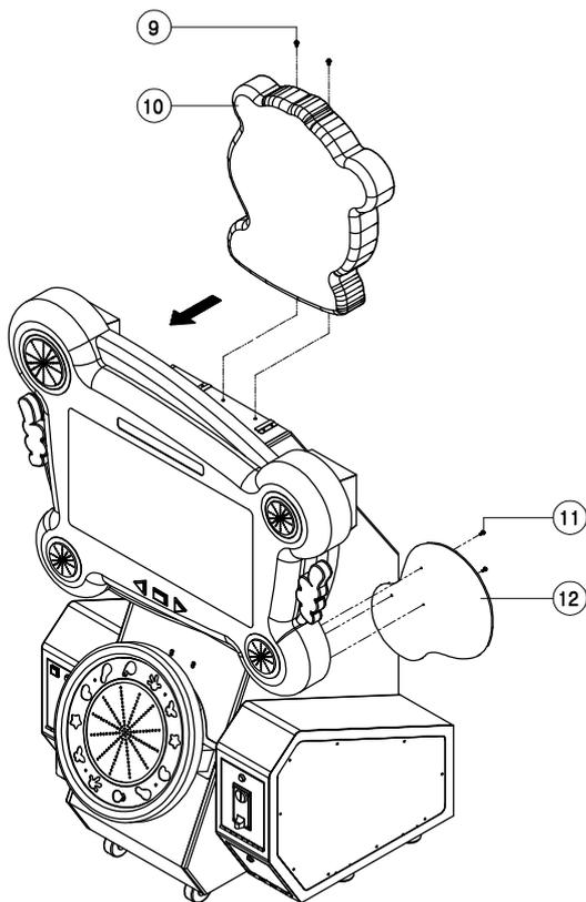
5. Attach ⑩ HEAD ASS'Y by using ⑨ M6x16L Bolts.(2 Bolts in total)
