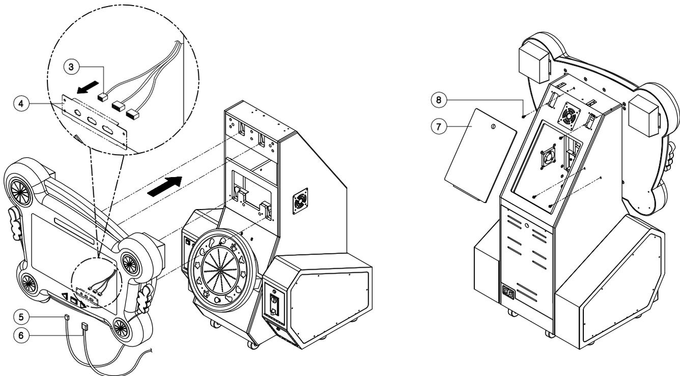
2. Open ⑦ the REAR UPPER DOOR and fix MASK ASS'Y using ⑧ HAND BOLT.
