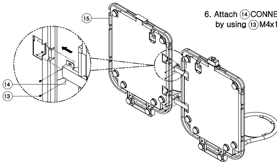
6. Attach ⑭ CONNECTOR BRACKET to ⑮ PUMP STEP ASS'Y R by using ⑬ M4x16L Bolts.(4 Bolts in total)
