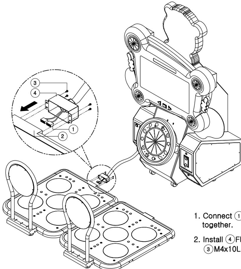
1. Connect ① MAIN CONNECTOR and ② STEP CONNECTOR together.
