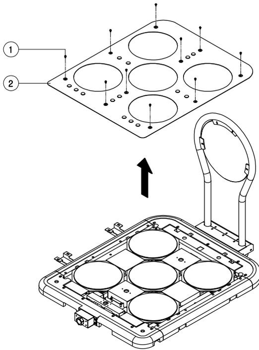
1. Release ① the Bolts then separate ② FOOT COVER BRACKET from the PUMP STEP ASS'Y.
