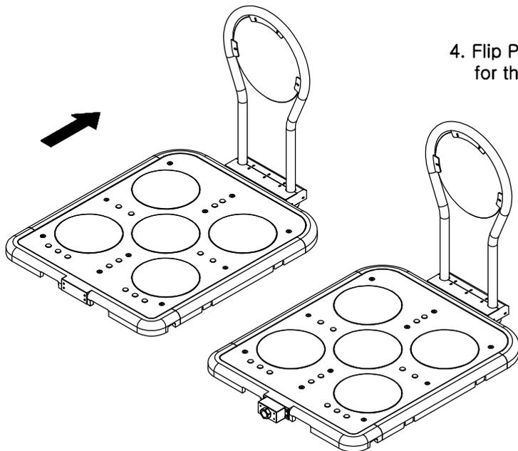
4. Flip PUMP STEP ASS'Y to see the bottom part of the ASS'Y for the next installation step.
