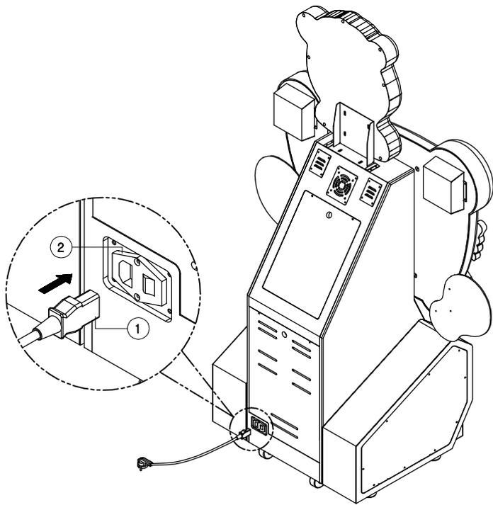
1. Insert Connect ① POWER CABLE to ② AC INPUT ASS'Y.
