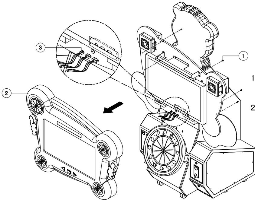
1. Detach (2) MASK ASS'Y by losing (1) M6x16L Bolts (7 Bolts in total)
