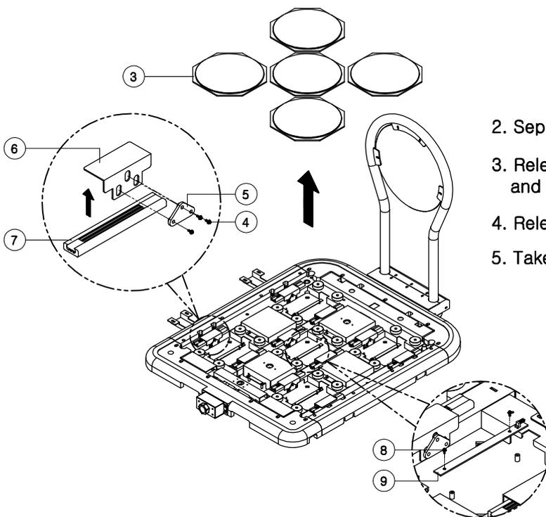
2. Separate ③ FOOT PLATE from the PUMP STEP ASS'Y.
