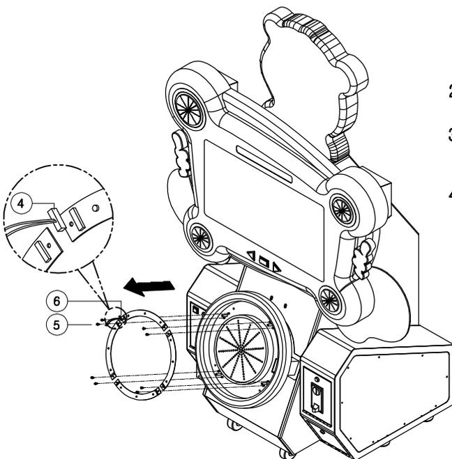
2. Detach ④ CONNECTOR from ⑥ WOOFER LED PCB.
