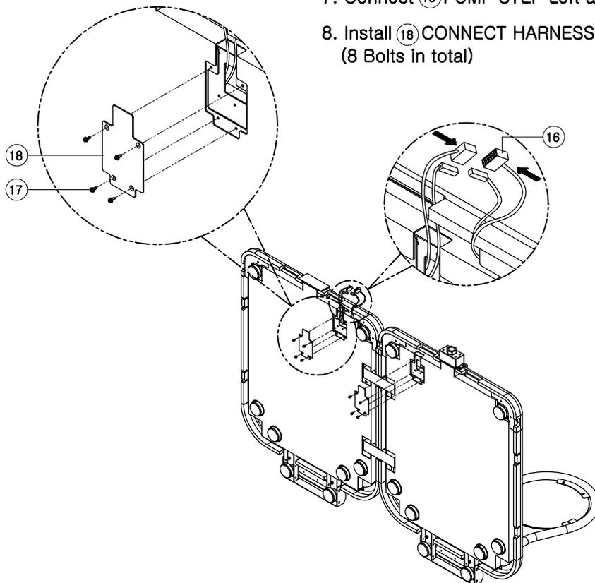
7. Connect ⑯ PUMP STEP Left and Right CONNECTOR together.
