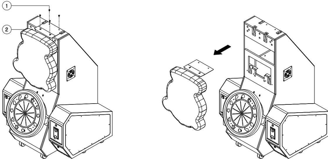
1. Detach ② MASK ASS'Y by loosening ① HAND BOLT.(4 Bolts in total)
