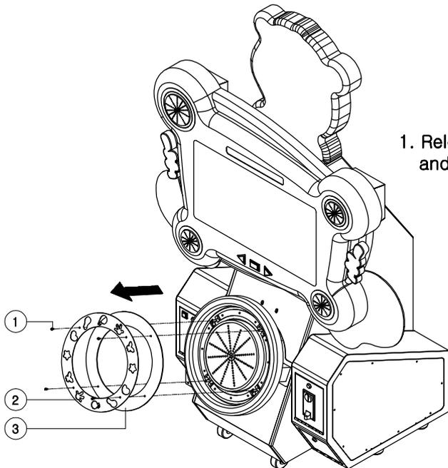
1. Release ① the Bolts then separate ② WOOFER CIRCLE BRACKET and ③ WOOFER CIRCLE PLATE ACRYL from the Main Cabinet.
