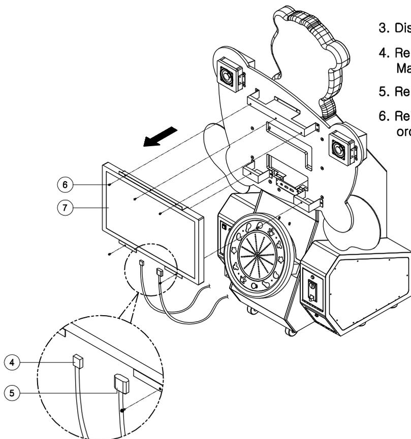
3. Disconnect (4) POWER CABLE and (5) MONITOR CABLE.
