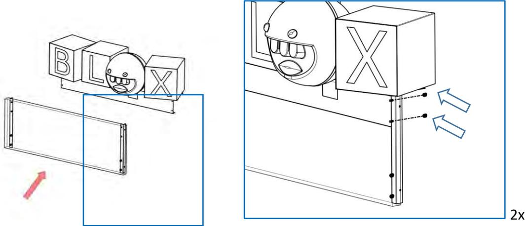
**10)** Install the header assembly with the upper side panels and Philipps 10-24 x 1¼ bolts
