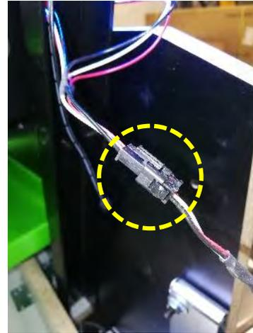
**12) L/H:** Plug the 3 power cables into their inputs and the LED Controllers together
