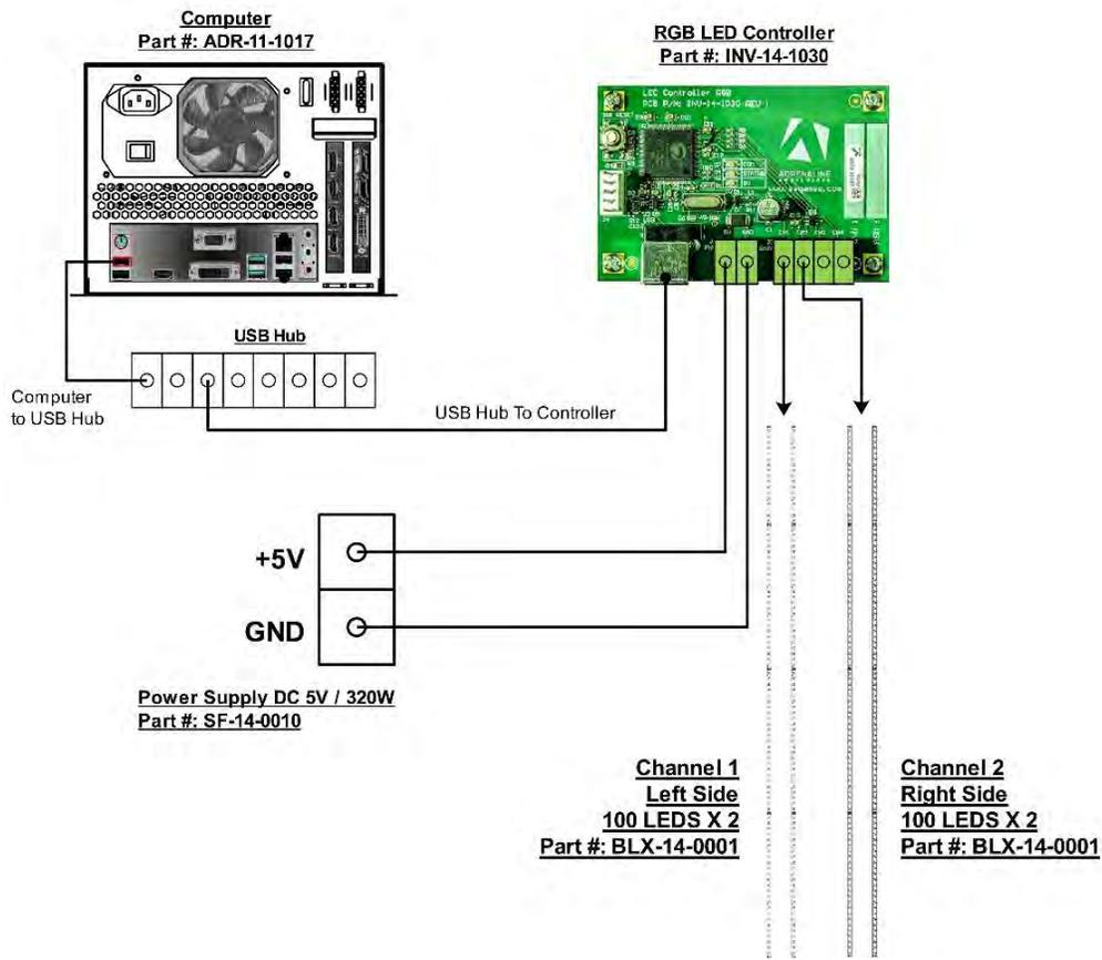
Each side has 2 strips of RGB PCB LED assembly
