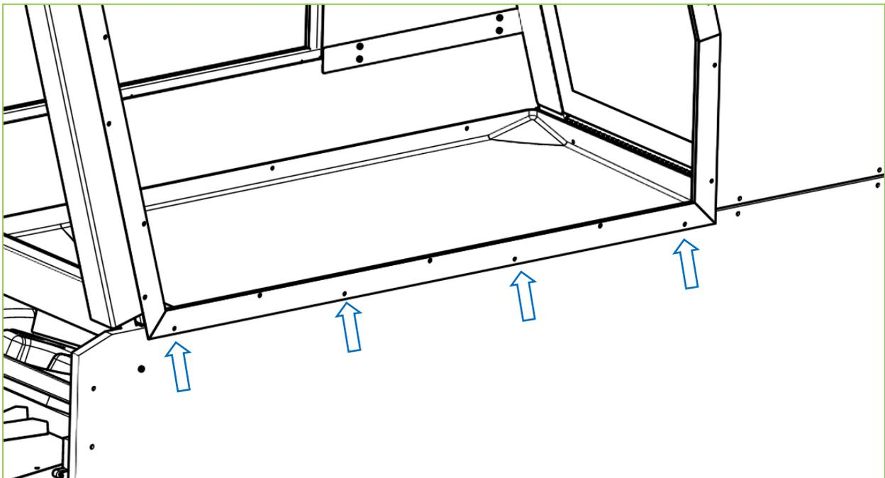
**9)** Assemble the header assembly and top display using Philipps 10-24 x 1¼ bolts for each side
