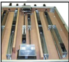
Playfield is supported on all 4 sides of the cabinet, by 2 beams running between the rods, and the tops of the player gear boxes.
