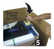
With the 5/8" Socket Wrench, loosen and remove the 2 Leg Bolts on each side of the front cabinet.
