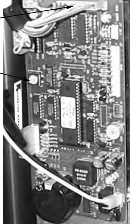
**NOTE:** when plugging in wire harnesses after servicing, be aware that the side of the wire harness plug that shows silver connectors always face the outside edge of the circuit board or see below for color chart.
