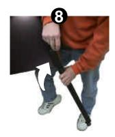
8. Using supports or two (2) people, prop the rear of the cabinet up and install **REAR LEGS**. *Secure tightly.*
