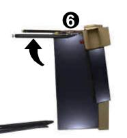
Install FRONT LEGS using the bolts removed from Step 4. Secure tightly. Take care not to scratch the Black Finish on any of the Legs.
