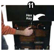
11. After the **BACKBOX** is in the **UPRIGHT POSITION**, locate the **5/16**" **HEX KEY**. While inserted, rotate **KEY** with a **3/4** turn until latched & locked.
