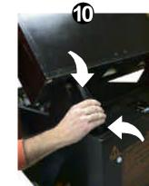
10. Lift the Backbox into the UPRIGHT POSITION (Ensure the cables do not get pinched).
