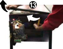
13. Open the Coin Door and pull the YELLOW HANDLE to the LEFT and at the same time pull up on the FRONT TOP MOLDING and remove. The
