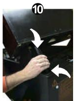
10. Lift the Backbox into the **UPRIGHT POSITION** (Ensure the cables do not get pinched).
