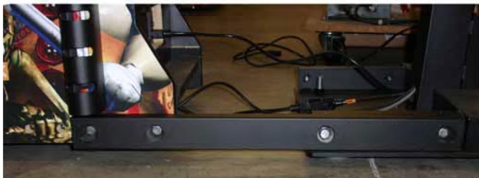
Mounting Bracket in Installed Position
