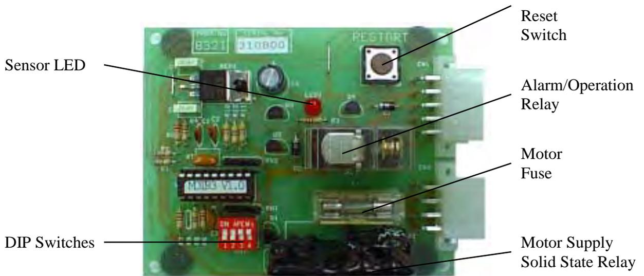
When the system operates and stops the motor, the supply to the motor remains off until manual reset is initiated. This creates the opportunity to ensure the machine is in a safe state to re-start; a visual check by the attendant ensuring that there is no longer any item causing the obstruction. Reset of the system is done by depressing the 'Restart' switch on the Motor Control PCB or by way of the remotely located reset switch (mounted on a T-board in the rear of section one).
