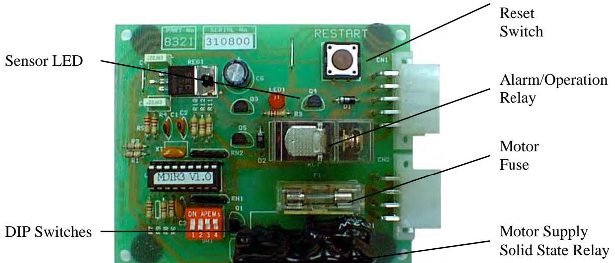
When the system operates and stops the motor, the supply to the motor remains off until manual reset is initiated. This creates the opportunity to ensure the machine is in a safe state to re-start; a visual check by the attendant ensuring that there is no longer any item causing the obstruction. Reset of the system is done by depressing the 'Restart' switch located on the roof, to the LH end of the top sign crest, section 1.
