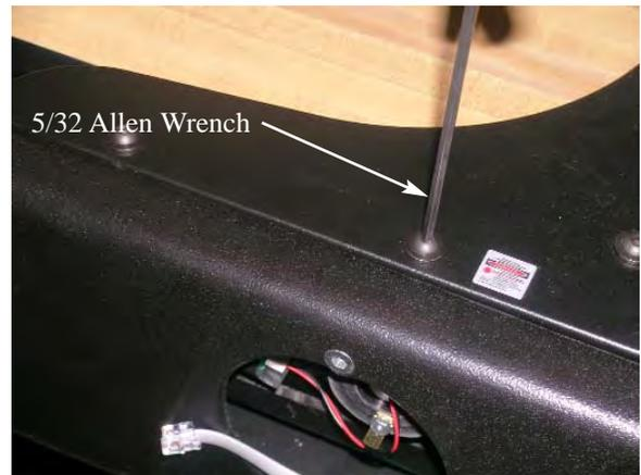
7. Insert the new module. There are alignment pins in the top of the sensor module. Use those to place the sensor module in the correct position.
