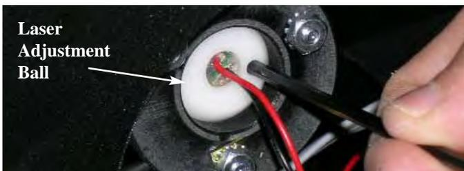
3. Insert the same allen wrench you used in step 1 into the hole provided on the laser adjustment ball.
