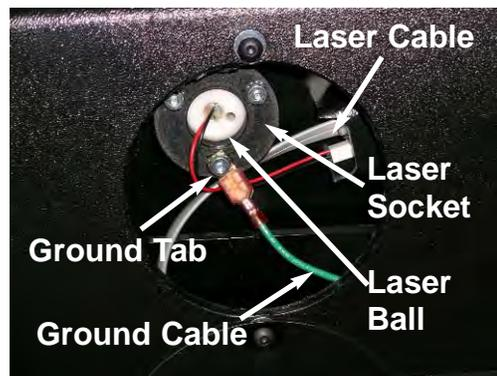
6. Remove the first half of the bracket by pulling it toward you. The laser will come out with it. Take note of how the bracket came out, you will have to put the new one in the same way.
