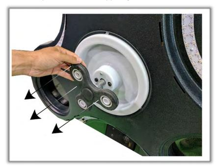
• Unscrew and remove the Values cover all around the Large Spinner.
