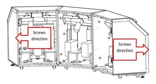
**2)** Between each dash's front, install metal part HTW-01-0009 (2x) with Philipps 10-24 x <sup>3</sup>/<sub>4</sub> machine screws
