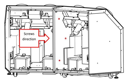
**2)** Between each dash's front, install metal part HTW-01-0009 with Philipps 10-24 x <sup>3</sup>/<sub>4</sub> machine screws
