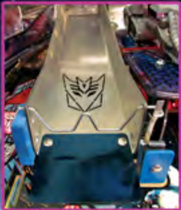
"Decepticon" laser-cut steel ramp.
